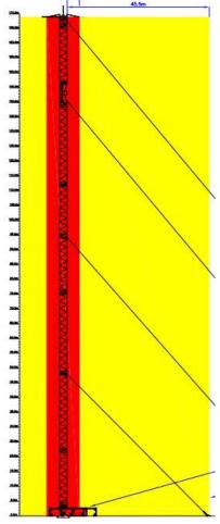
To the left is an example of an AM broadcast structure elevation view showing red and yellow zones. As you can see the whole structure is a red zone when operational.
