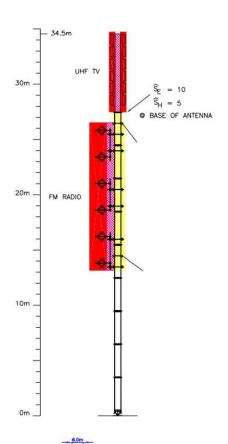
Here is an example of a TV / FM broadcast structure showing red, crosshatch and yellow zones. All of the EME is on the structure and the rest of the site has no eme exclusion areas.
