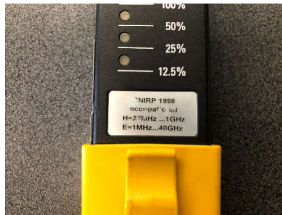
Typical RF Monitoring Device depicting Exposure Reference Standard set within unit E and H field range information on label
