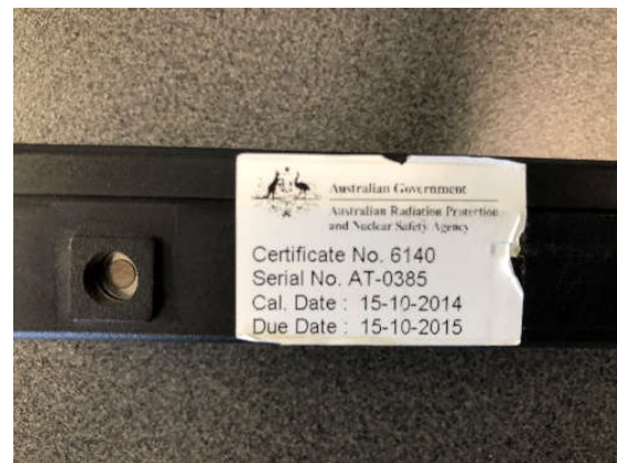
Typical RF Monitoring Device indicating Calibration label
